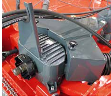
Splitter gearbox 290 hp rating - oil capacity: 1.00 gallon (3,8 liter)
