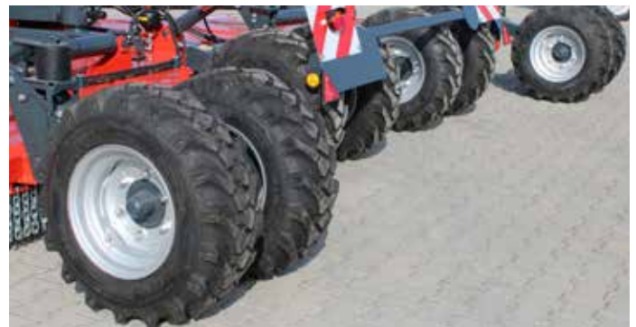
Various wheels and tires configurations including laminated, aircraft and pneumatic (depending on markets).
