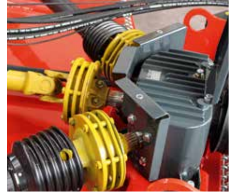
Secondary drivelines with 2-disc slip clutch each.
