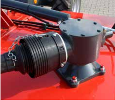
Rotor gearbox 180 hp rating - oil capacity: 0.92 gallon (3,5 liter)
