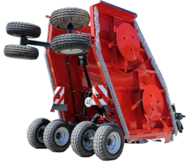
CONDOR 7300 ready for road travel, with optional 8 wheels (pneumatic) and optional 6-blade system.
