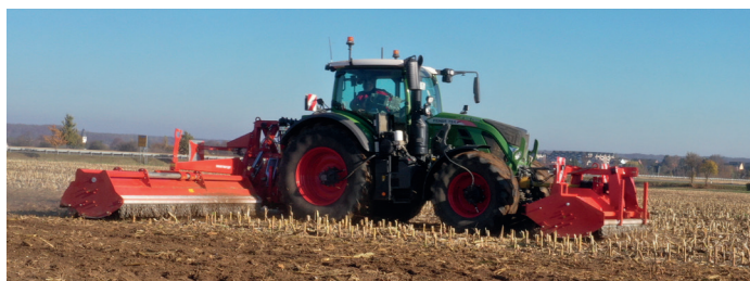
Split version: side mulching heads rear-mounted and center unit front-mounted
